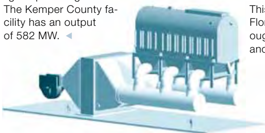
▲ DRYING OF LIGNITE. Fluidized bed dryer for the IGCC power generation facility in Kemper County, USA.
