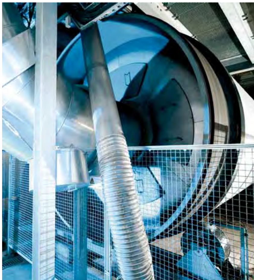
▲ ECO-FRIENDLY. Drum dryer for the eco-friendly production of high-grade granulate from sewage sludge.
